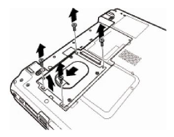
Figure 4-4 Removing 4 screws securing HDD assembly
